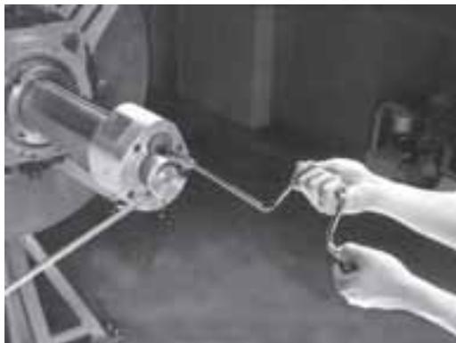
Manually adjusting the boring head position.
