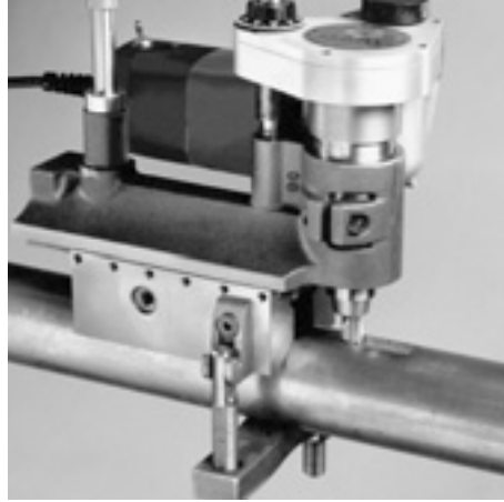
MOUNT IN MIDDLE The machine can be leveled for cutting long keyways.
